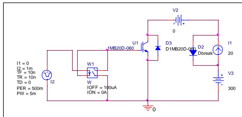
Test condition: Vcc=300 (V), Ic=20 (A), Vge=15 (V)
