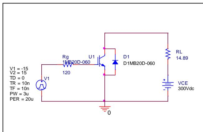
Test condition:  $I_C=20$  (A),  $V_{CC}=300$  (V)
