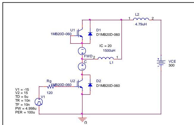
**Test condition:** Vcc=300 (V), IC=20 (A) –di/dt=60 A/usec
